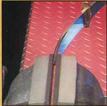
The Carbon V® Trailmaster® under extreme pressure at about 23° of torque. This blade returned to true after over one hour in this position. Most knives shatter or permanently bend well before they reach this point.
