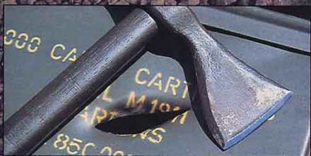
Above left, Lynn Thompson used the blade of the Vietnam Tomahawk to shear effortlessly through this heavy gauge ammo container, with no damage to the edge. On the right, you can see the Vietnam Tomahawk's spike punched through 3/4" plywood.
