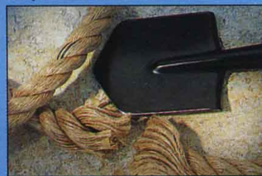
Above, Lynn Thompson takes aim with a specially sharpened shovel and severs a 1 1/4" manila hemp rope in a single stroke.
