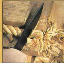
Manila rope is very tough on a knife edge. Its exterior repels all but the sharpest edges while its interior is abrasive enough to dull even the finest custom knives. Edges that can repeatedly cut this rope will last indefinitely under normal field use.
