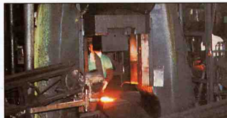
The red hot metal blank is placed on the anvil die.
