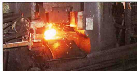
Above you can see the huge air hammer in action. As you can imagine the force is incredible as the softened, red hot steel is pounded into shape in the metal die. The entire building shakes as the hammer makes contact and the sound is deafening!
