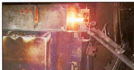
Above, a metal blank is heated in a furnace.
