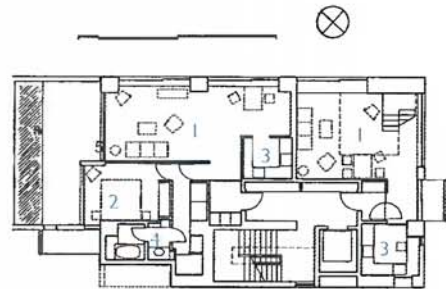
Fourth floor plan 1. Living Room 2. Bedroom 3. Kitchen 4. Bath 5. Roof Terrace 6. Closet 7. Living Room 8. Library
