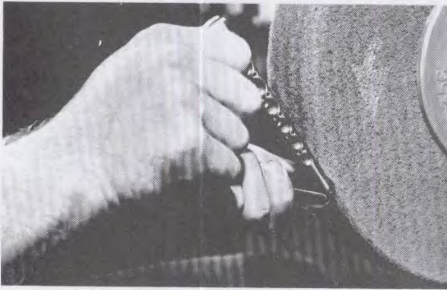
The scratches are removed from the tang slots and the outside handle backs.
