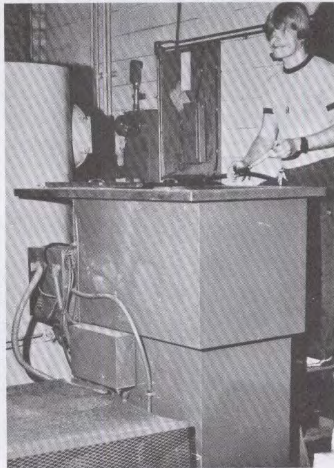
For a large volume of knives, this vapor degreaser can accommodate up to 2,700 pounds of metal.
