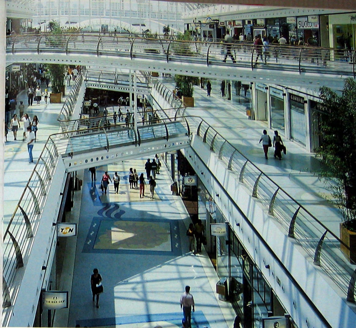
The rows of shops on the upper levels are dramatically connected by walkways – echoing ship gangways – made of glass slabs and curvaceous railings.
